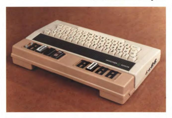
The ROMBOX enables Electron and BBC users to run ROM based software such as Slogger's STARMON Machine Code Monitor or STARWORD word processor. Robustly constructed and attractively designed, ROMBOX provides sockets for 8 ROMS which may be the usual 8k (type 2764) or 16k (type 27128), but user selectable options also enable 4k ROMS and RAMS to be used.
